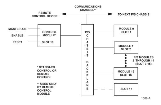
Figure 2-3. Control Module, Simplified Block Diagram (Standard and Remote)
